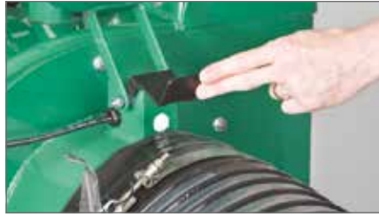
Safety Kill Switch Quick connect / release hose clamp with safety interlock.
